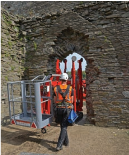
Figure 4 Mobile elevating work platform passing through doorway
